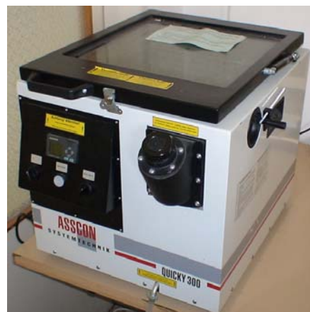
FIGURE 4: THE VAPOR PHASE SOLDERING DEVICE ASSCON QUICKY 300
