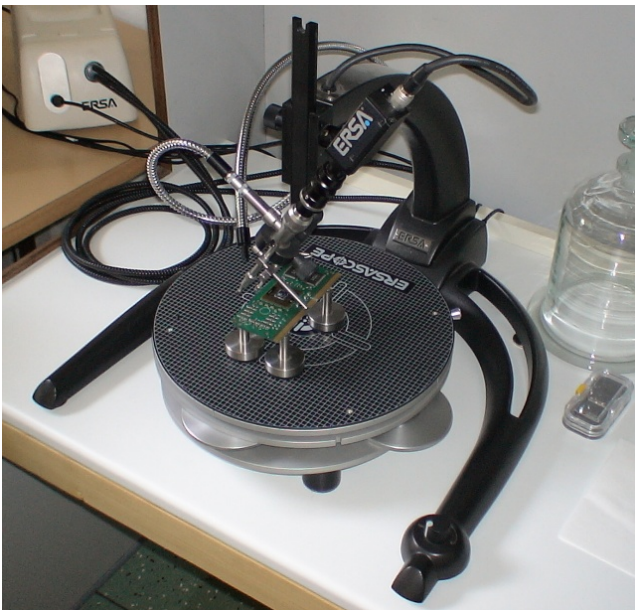
FIGURE 6: THE MODERN OPTICAL SYSTEM ERSASCOPE FOR FABRICATED SAMPLES SOLDER JOINTS VERIFICATION
